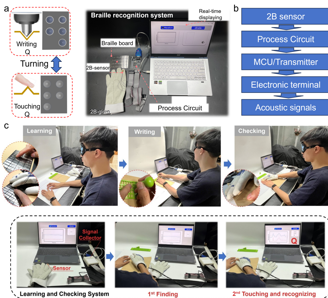
Figure 7 Intelligent interaction application scenario. (a) Schematic illustration of writing and touching Braille “Q”, and the photograph of the Braille recognition system including 2B-sensor, Braille board, process circuit and MCU. (b) The working process of the Braille recognition system. (c) Applications of the two-channel 2B-glove for learning, writing and recognizing Braille.
